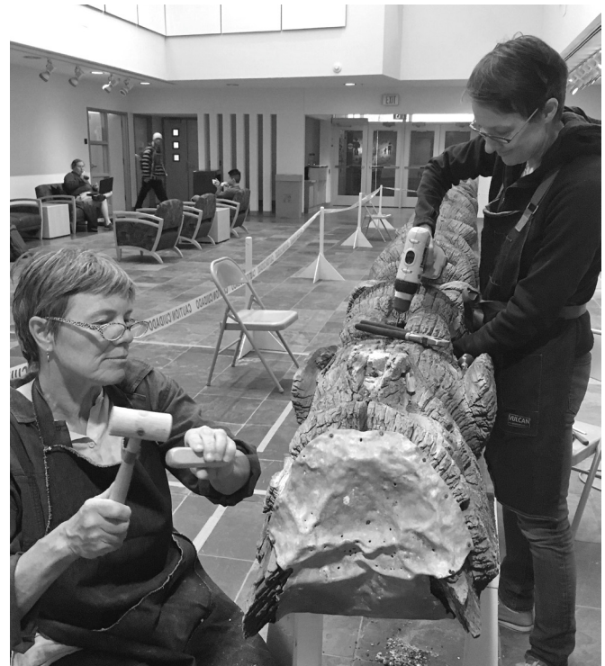
Figure 5. Conservators Rae Beaubien, left, and Mina Thompson drilling and chiseling out the fills. Note the metal cap, which obscures extensive plaster fill in the kingfisher's head. (Image courtesy of Landis Smith.)
