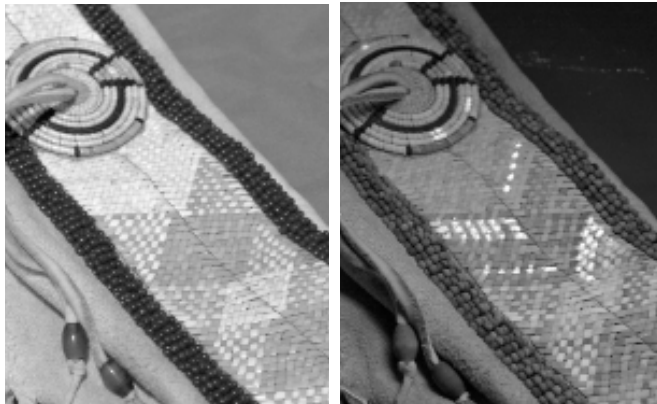
Quillwork repairs labeled with ultraviolet marker, shown under ambient light and 254 nm UV
